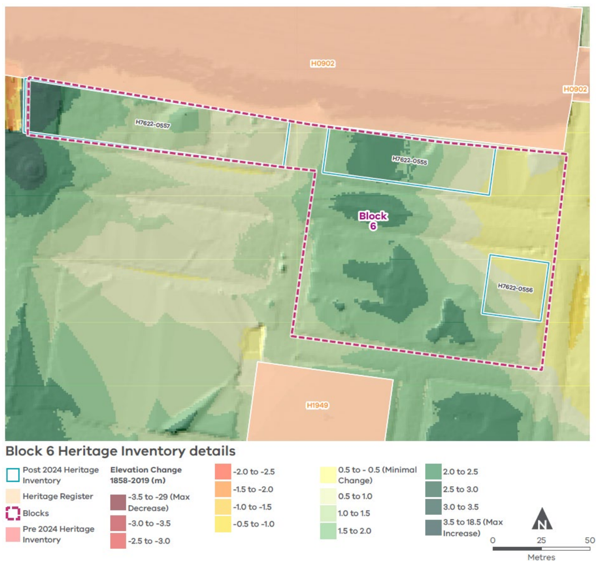
Figure 32: Plan showing the Digital Elevation Modelling indicates that across Block 6 ground levels likely increased by 2–2.5 metres, with Mair Street East almost certainly being raised.
