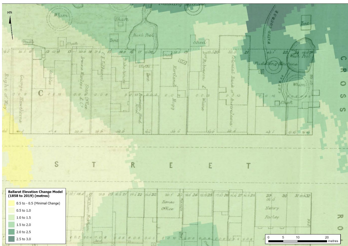
Figure 52. The elevation modelling over an 1857 map of Bridge Mall. Here, puddling machines and the Times Office are in locations predicted to have increased in elevation by at least 1.5 metres since 1858.
