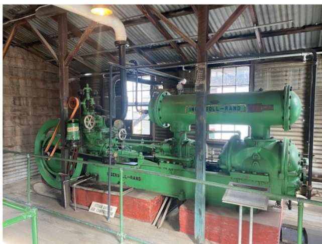
2025. Steam compressor and compressor house. Source; Bendigo Heritage Attractions.
