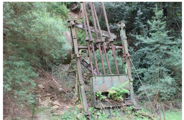
Figure 8. Five-head stamp battery relocated to Long Tunnel Extended Gold Mine Reserve (Peter Davies)
