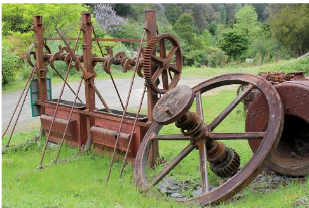
Figure 7. Ten-head stamp battery built by Langland's Foundry in Melbourne in 1888 and relocated to the Long Tunnel Extended Gold Mine Reserve from the Harbinger mine (Peter Davies)
