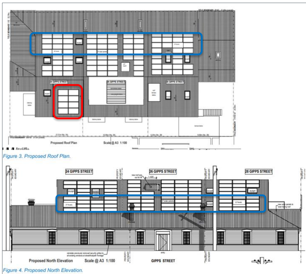
Figure 4. Roof plan and elevation showing solar panels in dispute, outlined in blue. Solar panels outlined in red, on the southern roof face, are not in dispute.
