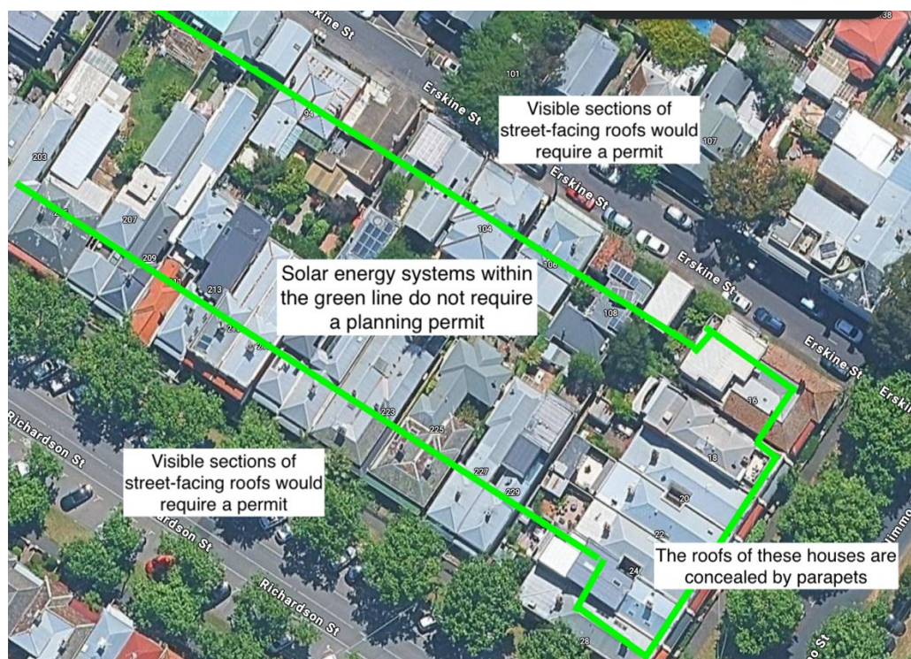
Figure 1: Example of non-publicly visible locations for solar installation in a Heritage Overlay area.
