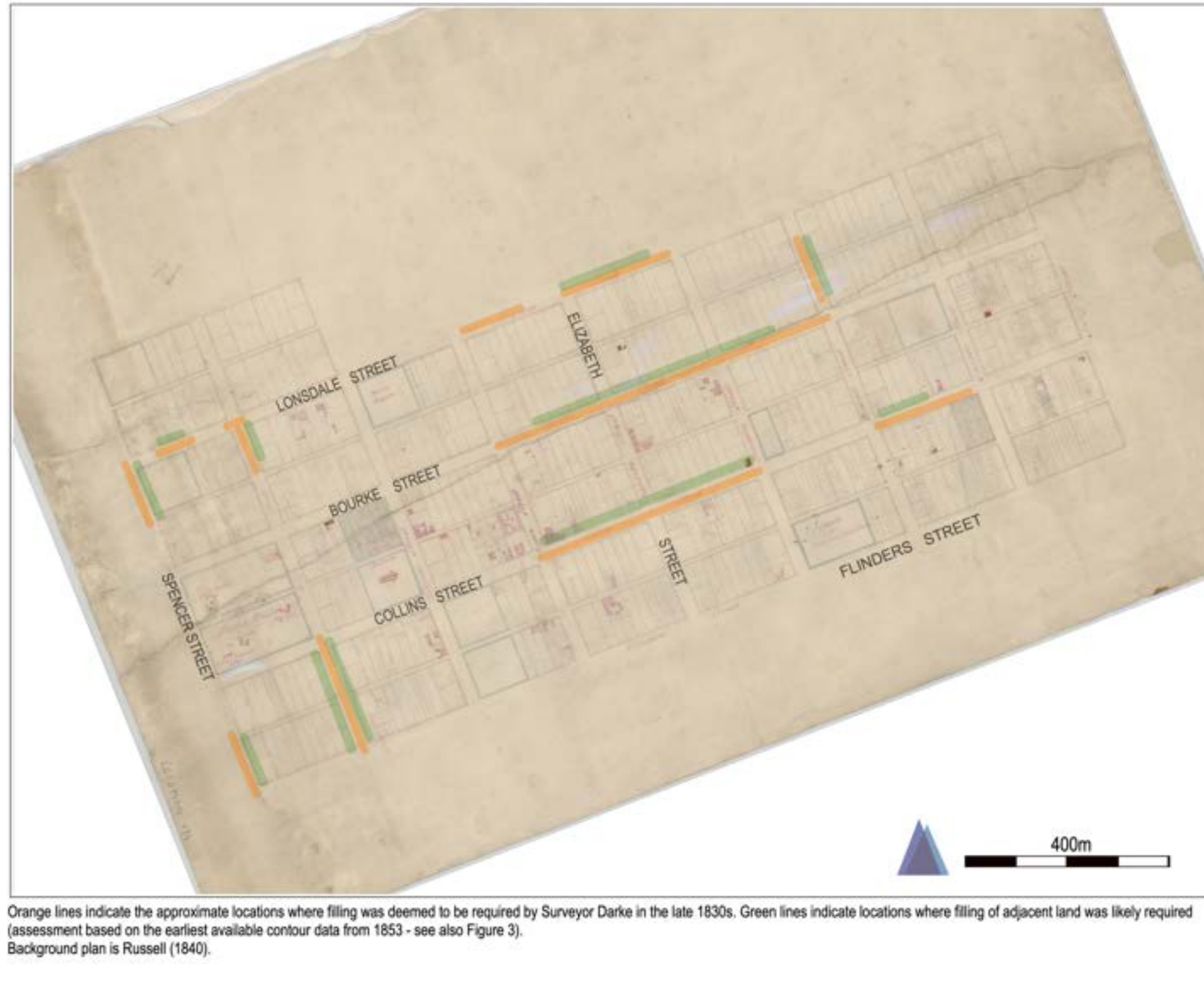
Figure 22 Preliminary assess of the likely locations that filling may have been required, based on Darke's 1837 proposed street levels (Figure 3) and the 1853 contour data.
