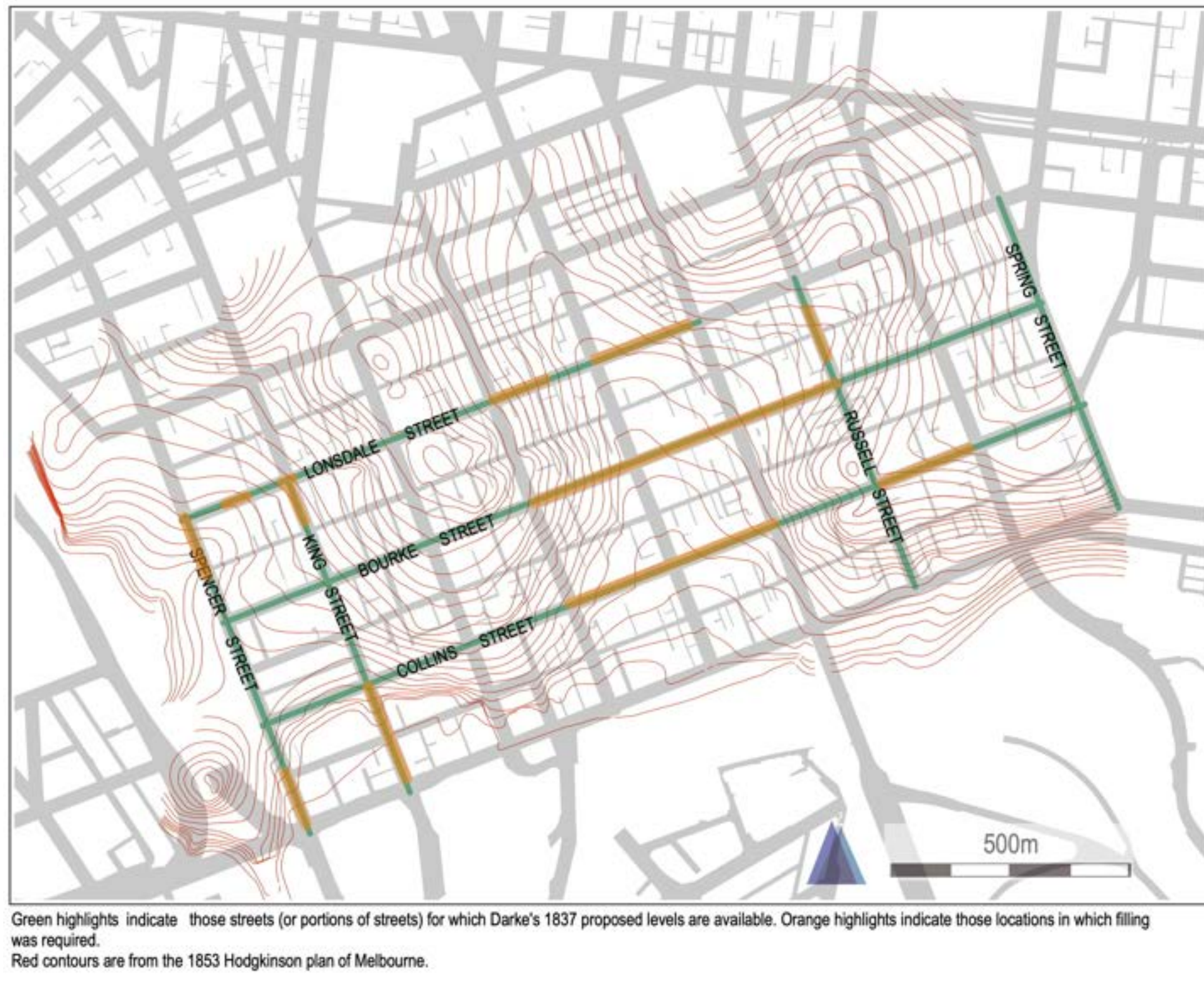
Figure 2 Plan of the Melbourne CBD, showing the streets for which surveyor Darke's 1837 proposed levels are available, and showing those locations where filling was considered to be required (in orange).
