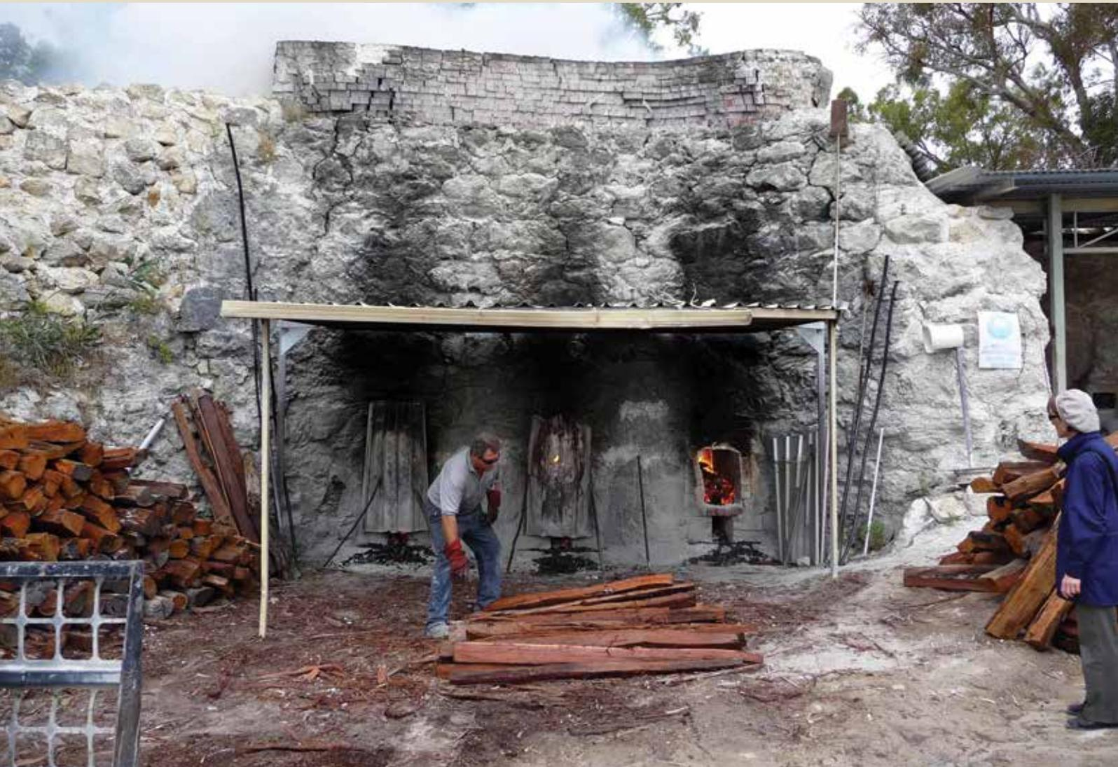
**Figure 7: Traditional lime burning.** A lime kiln at Susac Lime Supply, Carabooda, north of Perth, Western Australia. This may be the last such lime kiln operating in Australia: most had ceased production by World War II.
