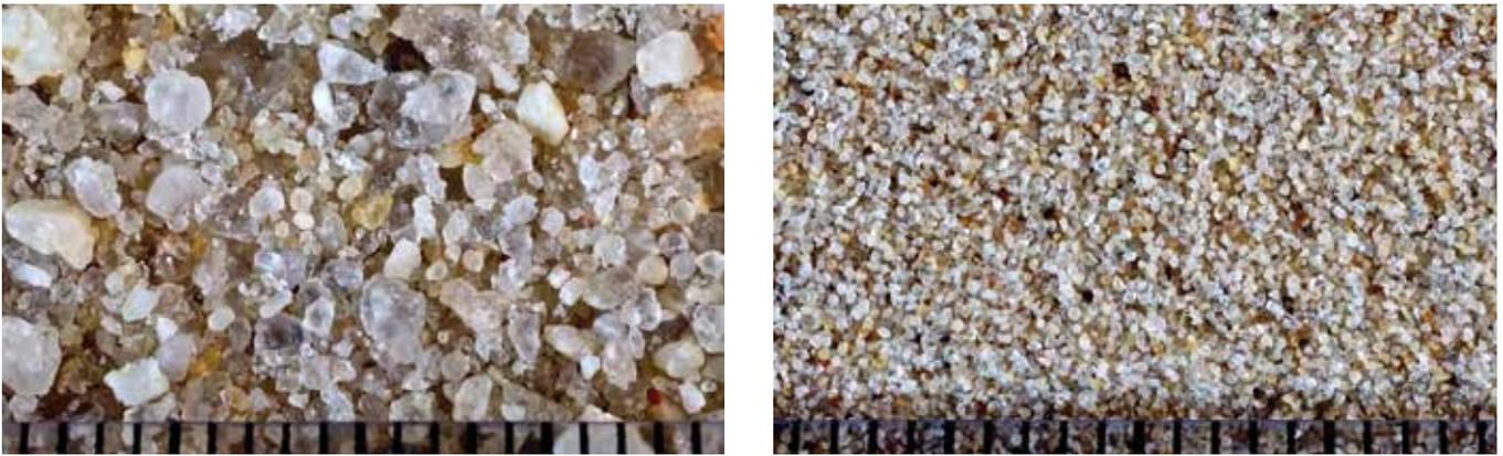
**Figure 19: Grading of sands.** The sand on the left is well graded. It has a wide range of particle sizes from very coarse through coarse, medium, fine and very fine. The sand on the right is poorly graded, with a relatively uniform (fine to medium) particle size. Each division on the scales in these photographs is 1 mm; each image is about 20 mm across.
